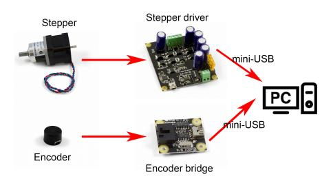
Figure 6: Connection logic of stepper and encoder
