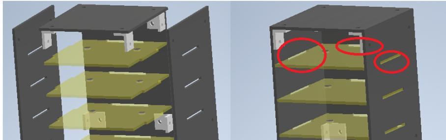
Figure 16: New design of arena platform connection
