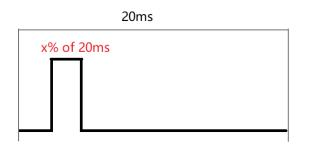
Figure 14: Manually generated PWM pulses
