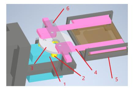
and is pretty easy to control. For the movement conversion a Scotch-yoke mechanism is considered.
