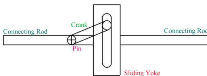
Figure 10: Scotch-yoke mechanism
