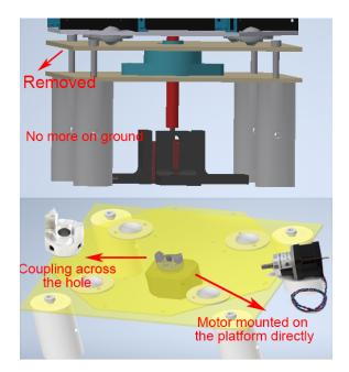
Figure 5: Coupling of the carousel platform of the old and new version of Optobot
