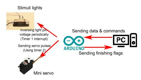
Figure 12: Control logic of the Arduino
