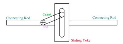
Figure 10: Scotch-yoke mechanism
