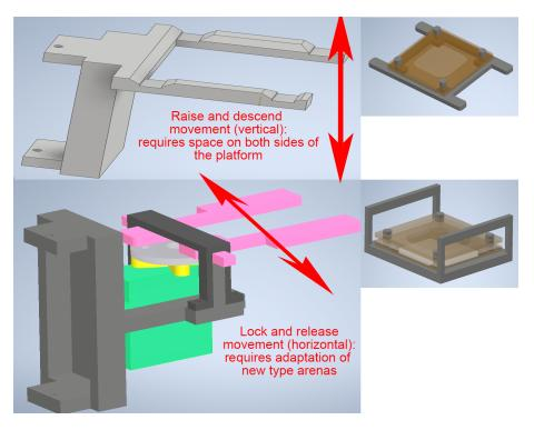
Figure 8: Comparison of the old and new gripper design
