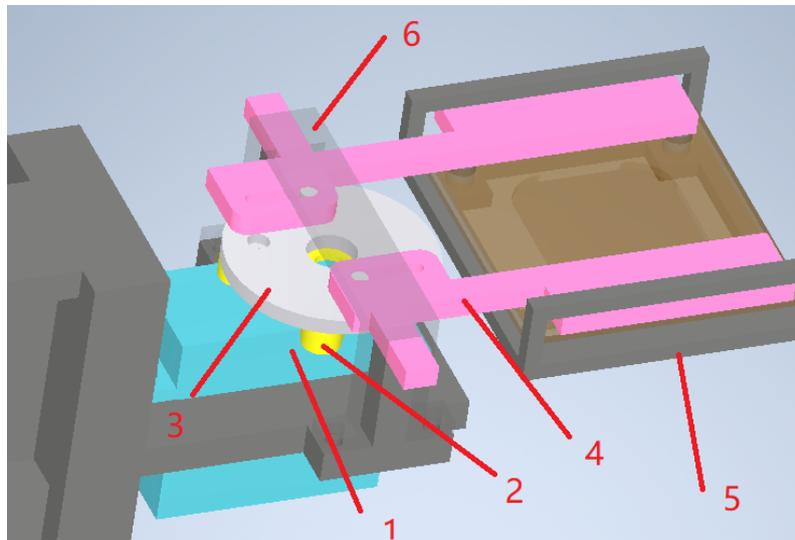
Figure 9: Mechanical design of the gripper
