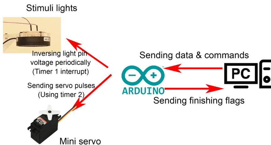
Figure 12: Control logic of the Arduino
