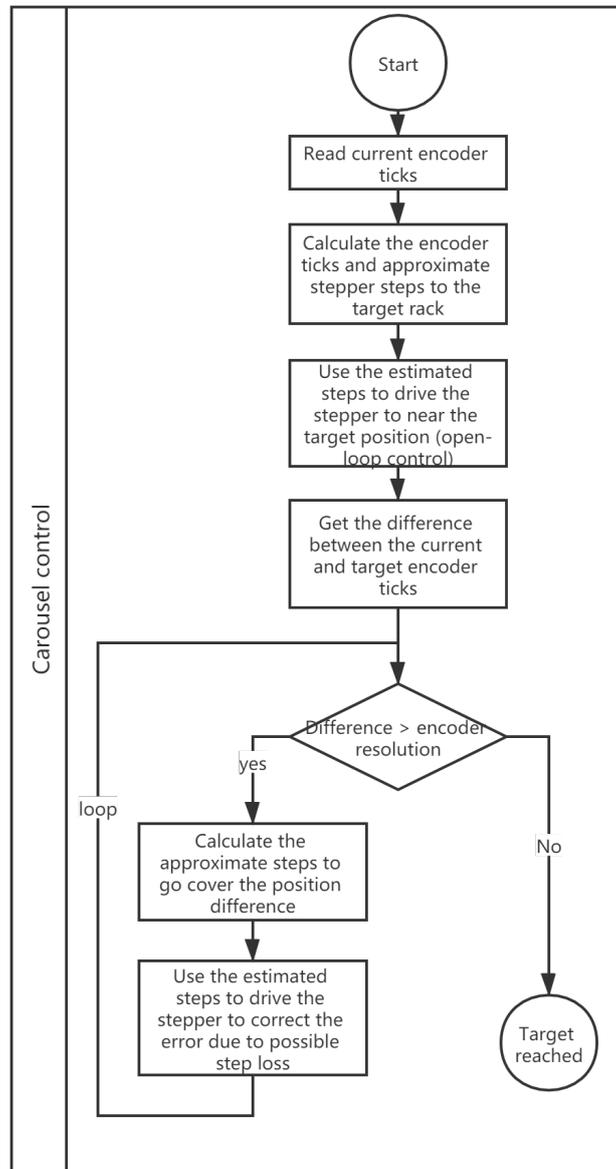
Figure 7: Connection logic of stepper and encoder
