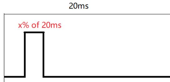
Figure 14: Manually generated PWM pulses
