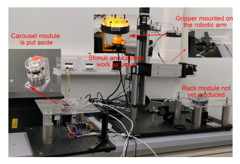
Figure 20: Setup of overall test
