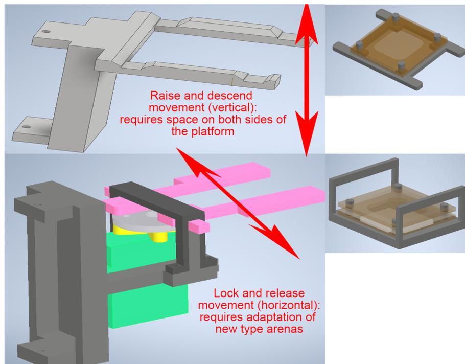
Figure 8: Comparison of the old and new gripper design
