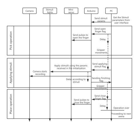
Figure 13: Communication graph of the Arduino
