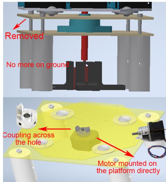
Figure 5: Coupling of the carousel platform of the old and new version of Optobot
