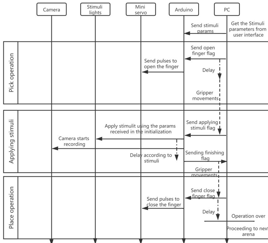
Figure 13: Communication graph of the Arduino
