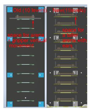
Figure 17: Comparison of the rack capacity in the old and new design
