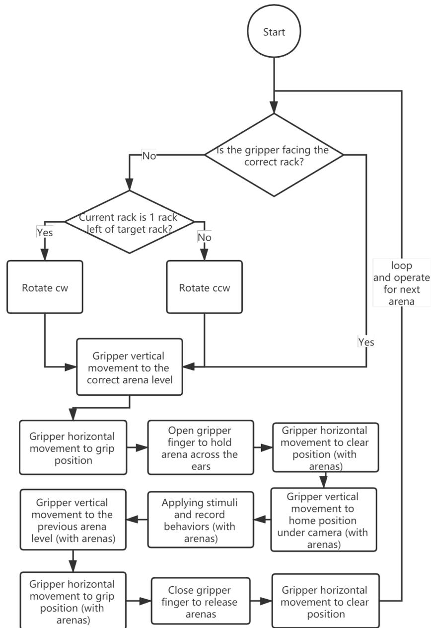
Figure 3: System events for single arena operation
